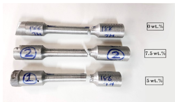
Fig. 9. Tensile specimens after testing.
